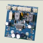
The Keyscan DPS-15 is a dual-linear DC power supply with two outputs for ACU-12VDC at 1.2 Amperes and AUX/RDR-12VDC at 1.2 Amperes.
