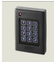
Farpointe Data single-gang mount Indala format proximity surface mount keypad reader. Dual reader and keypad. Wiegand output. Reads the Keyscan 125 kHz 36-bit Indala format. A HID PXK501 replacement reader. Black. 18" (457.2 mm) – 9 conductor shielded cable pigtail. Two-piece design with snap-on cover to hide mounting screws. Weight is 4 oz (113 g). Product Listings: UL294, FCC, IC. Warranty: Limited Lifetime.
