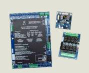
The Keyscan CA250NB is a network appliance-based access control unit that gives you unmatched flexibility for new installations or revitalizing aged or failing access control systems. The CA250NB is a package that includes 1 CA250B ACU board, 1-OCB8 relay board, and 1-DPS-15 power supply. This does not include a black metal enclosure.
