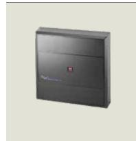
The Farpointe P-900-H reader is a long range reader solution ideal when long-range read applications are required. Fully supported by Keyscan and other access control systems the Farpointe P-900-H offers up to 20" read range and is a cost effective alternative to other traditional 125 kHz technology readers. Available Black only. This reader will require additional 12VDC power supply.
