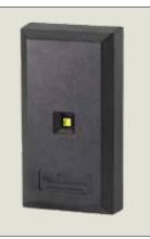
Farpointe Data mullion mount Indala format proximity surface mount reader. Wiegand output. Reads the Keyscan 125 kHz 36-bit Indala format. A HID PX-603 replacement reader. Black. 18" (457.2 mm) – 9 conductor shielded cable pigtail. Two-piece design with snap-on cover to hide mounting screws. Weight is 3 oz (85 g). Product Listings: UL294, FCC, IC. Warranty: Limited
