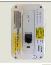
An E-Plex Gateway provides two-way communication from an E-Plex Lock to Keyscan Aurora software. A Gateway communicates to Aurora by a direct connection to a USB (non-network) or TCP/IP network. A Router acts as a repeater, extending the radio frequency (RF) communication between the Gateway and E-Plex Locks.
