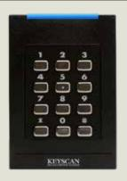
iCLASS® Seos Only Profile Single gang or wall mount keypad reader. Only supports the new Seos® technology physical and HID mobile credentials. Not backwards compatible with iClass SE or iClass Legacy physical credentials. Highly secure and ready to support HID NFC and/or BLE Mobile Access®. Requires on-boarding process to obtain Mobile credentials. Contact Keyscan for further details. May require plastic spacer for mounting on metal. Available black only.
