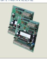
When circumstances dictate a long cable run between control panel and reader, exceeding 500 feet, rely on the Keyscan WIEEX2 wiegand extender. This interface converts the Wiegand signal to standard RS485 providing a communication range of up to 4000 feet between WIEEX2 receiver and WIEEX2 transmitter while using standard CAT5 cable between units.
