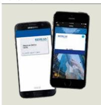
LEGACY 36-Bit format mobile credential for use with K-SMART3 reader. These credentials are designed to be used with specific Aurora software platforms and requre an RSA software key to develop. Due to that technical nature these legacy Mobile credentials will only be available direct from Keyscan
