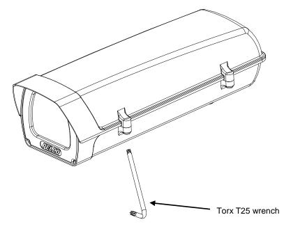
Remove the camera plate. Install the camera on the plate and tighten screw.
