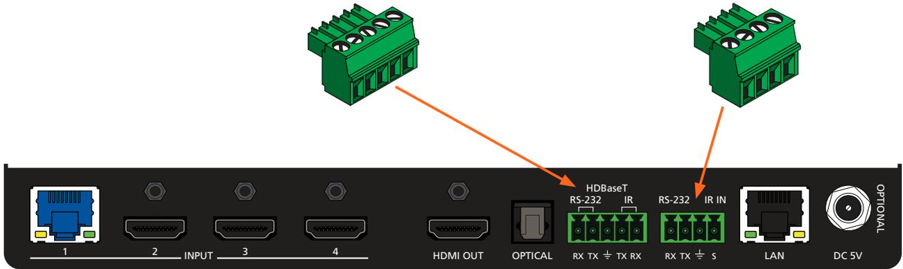
1. Locate the required captive screw connector (included in the box).
