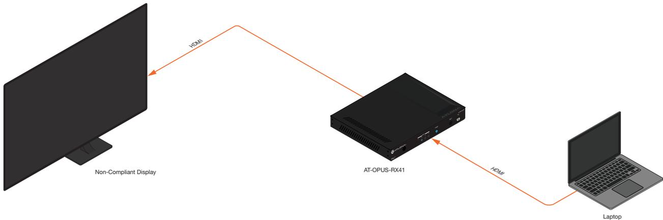
By default, the laptop may transmit HDCP content. However, when connected to a display that does not support HDCP, the laptop must be instructed to send non-HDCP content, in order for the content to be displayed.
