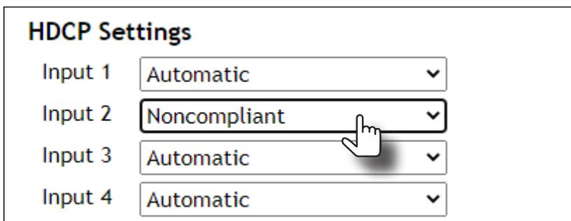
**i NOTE:** Not all source devices are capable of transmitting non-HDCP content. For example, Sony PlayStation® gaming consoles and Mac® computers always transmit HDCP-encrypted content.
