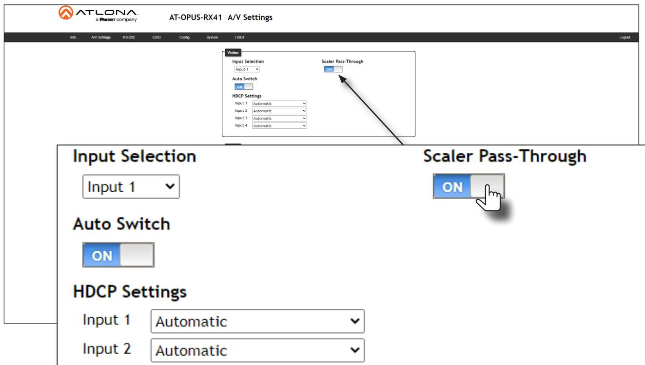
4. Click the toggle switch again, to return the **Scaler** toggle to the **OFF** (default) position, and allow downscaling of 4K content.
