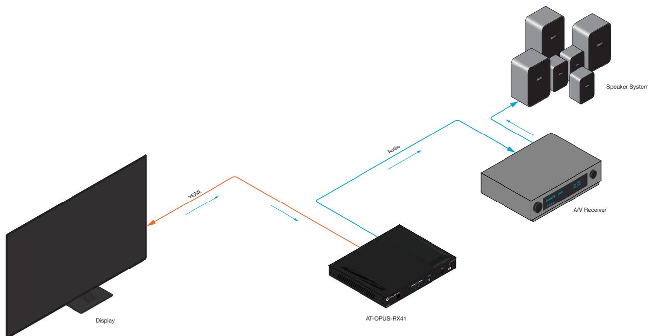
1. Connect an HDMI cable from the **HDMI OUT** port on the AT-OPUS-RX41 to the HDMI input port on the display. This cable is used to carry the audio from the display to the AT-OPUS-RX41.
