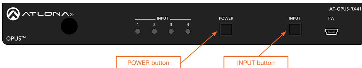
3. Press and hold the **INPUT** button on the front panel for approximately 20 seconds. Release the **INPUT** button once the **POWER** button begins to flash blue and red. The number of flashes will indicate the currently selected IP mode.
