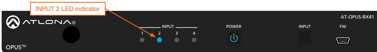
2. Press the **INPUT** button again to switch to **INPUT 3**. Once INPUT 4 is selected, and the **INPUT** button is pressed again, the unit will return to **INPUT 1**.
