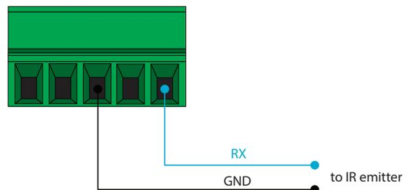
*Figure 2.3 - Wiring the 4-pin HDBaseT RS-232/IR IN captive screw block to control the AT-OPUS-RX41 over IR.*
