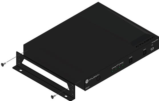
4. Mount the unit to a flat surface using the oval-shaped holes, on each mounting bracket. If using a drywall surface, a #6 drywall screw is recommended.
