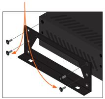
To provide added stability to the mounting bracket, use two of the included screws and attach them to the two holes, directly below the enclosure screws, as shown above.
