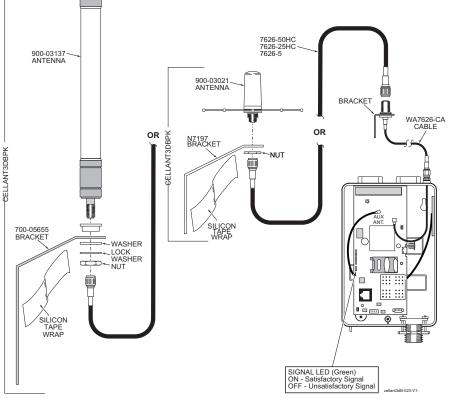
Figure 1 – CELLANT3DBPK Remote, Weatherproof Antenna
