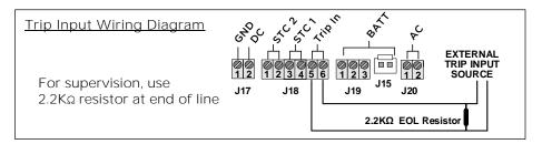
NOTE: Be sure to use a UL-approved 2200-ohm resistor if the trip input circuit will be supervised (e.g., Bosch P110BL, Bosch EOL-22K, Elk ELR 22). The trip input circuit is not supervised for ground conditions.
