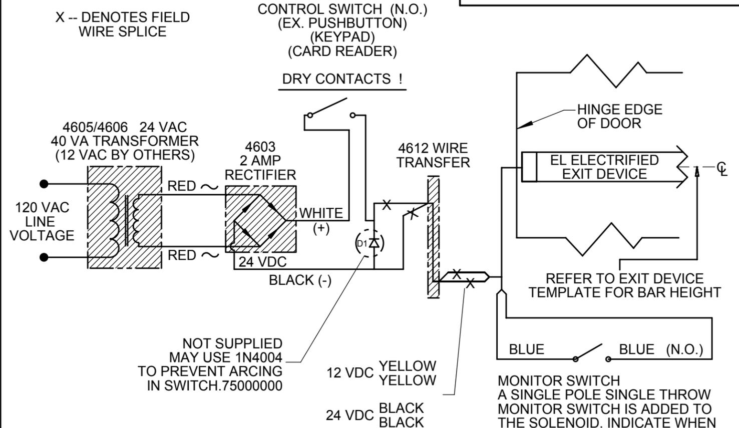
FIG. 1 ELECTRIC LATCH RETRACTION WIRING SCHEMATIC
