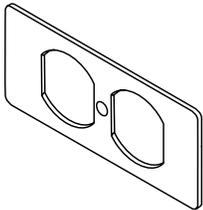
**Duplex Receptacle Faceplate** – For covering duplex style devices. Also accepts 106 communications frame.
