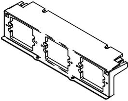
**Mounting Bracket** – Holds up to three (3) devices of power, communications or A/V devices. Bracket accepts standard size (2 3/4" x 4 1/2" (70mm x 114mm)) device plates sold separately by others.
