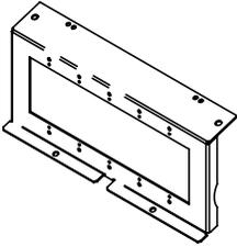
**Mounting Bracket** – Holds a standard 5 gang device plate
