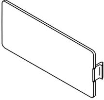
**Blank Faceplate** – For covering unused compartments in the device bracket.
