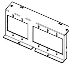
**Mounting Bracket** – Equipped with one 2-gang standard size device opening and one 3-gang standard size device opening. Accepts a standard 2-gang (4 9/16" x 4 1/2" (116mm x 114mm)) and a 3-gang (6 3/8" x 4 1/2" (162mm x 114mm)) device plate. Ideal for 2-gang A/V devices such as Crestron® 2-gang and 3-gang digital media devices. Device plates and devices supplied by others.
