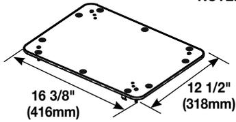
**NOTE:** Ring must be attached to the floor box before pouring concrete or terrazzo.
