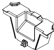
**Tunnel** – For EFB8 Series and EFB10 Series boxes. Tunnel allows cables to be wrapped around box from one module to the other.
