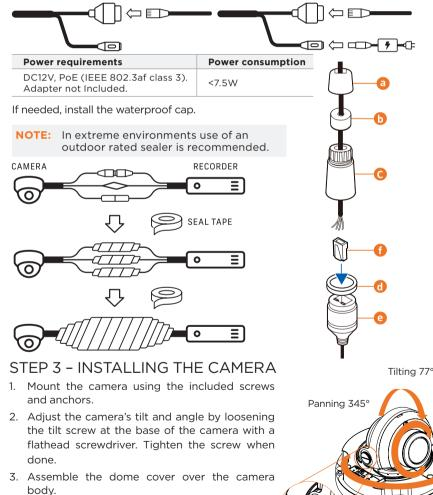
4. Remove the protective film from the dome. Softly wipe the dome with lens tissue or a microfiber cloth with ethanol to remove any dust or smudges left from the installation process.
