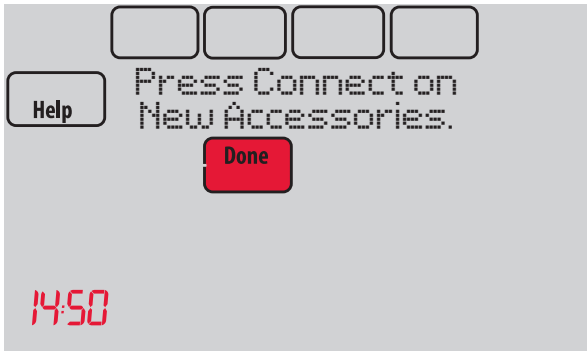
Fig. 35. Thermostat in listening mode.
