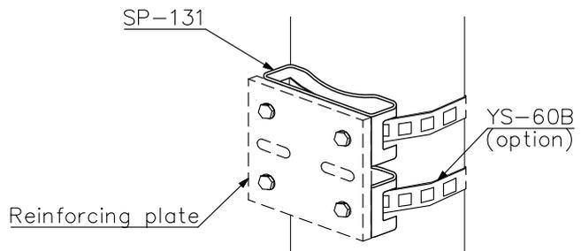
Example of mounting reinforcement
