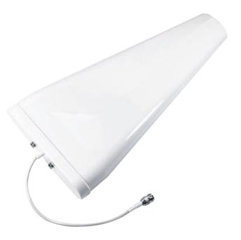
The TQ-230W is an outdoor yagi antenna that can be aimed in the direction of the closest cellular tower and pick up signals up to 30 miles away. The wide band yagi antenna is designed to cover 2G/3G/4G/and WLAN systems for Cellular, PCS, AWS and LTE frequencies.
