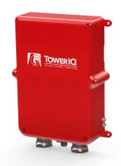
The TowerlinQ system consists of a set of active nodes each of which itself is a transceiver. The controlling node (the hub) and regular nodes, up to 40 of them, communicate to each other via a serial bus type signaling line of the total length up to 1000 m (can be extended with TQR repeater). In addition to the Hub and the Nodes, the system includes a DRC (Dedicated Radio Console) unit and is integrated with a supporting TIQ.Cloud application.
