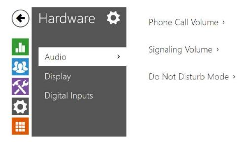
2N® Indoor View is equipped with a speaker. Set the phone call and state signaling volume control in this configuration section. Master Volume controls the general device volume including call volume, signaling tone volume, and so on. Consider the noise level of the ambient environment while setting this parameter.
