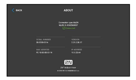
This section provides basic information on the device (serial number, MAC address, FW version, IP address, My2N ID).
