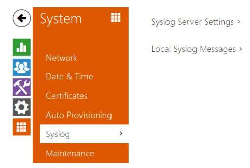
**2N** \*\* Indoor View allows you to sends syslog messages including relevant device state and process information to a syslog server for recording and further analysis or auditing of the device observed. It is unnecessary to configure this service for common operations.
