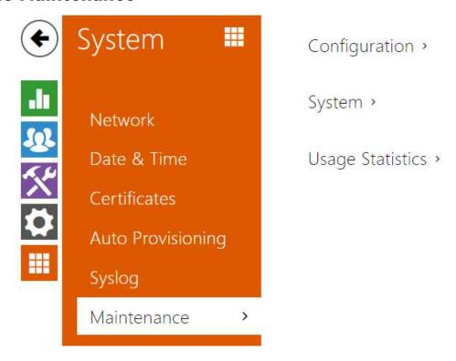
This menu helps you maintain the device configuration and firmware. You can back up and restore all the parameters, upgrade firmware and/or factory reset the device.
