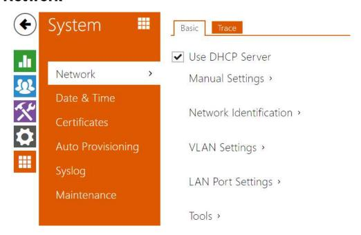
**2N** \*\*Indoor View is connected to the LAN and has to be assigned a valid IP address or obtain the IP address from the LAN DCHP server. The Network section helps you configure the IP address and DHCP.
