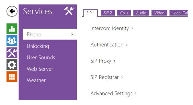
Phone is an essential function of  $2N^{\circledR}$  Indoor View allowing you to establish connections to other IP network terminals.  $2N^{\circledR}$  Indoor View supports the extended SIP.
