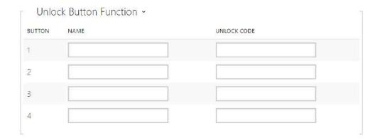
• Code 1, 2, 3, 4 - enter the code assigned to unlock button #1, #2, #3, #4. It is used for remote unlocking of the entrance door, for example. Make sure that the code includes at least two door unlocking characters via the intercom keypad and at least one door unlocking DTMF character via a phone. Four characters at least are recommended.
