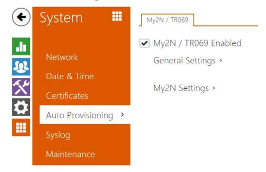
The  $2N^{\circledR}$  Indoor View help you update firmware and configuration manually, or automatically from a storage on a TFTP/HTTP server selected by you according to predefined rules.
