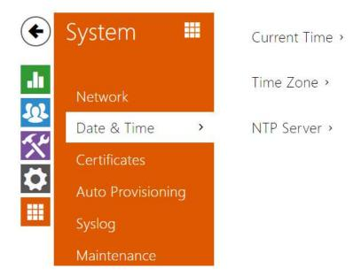
**2N**<sup>®</sup> **Indoor View** is equipped with a real time clock to back up the device for even a few days in case of power outage. Click **Synchronise** to synchronise your **2N**<sup>®</sup> **Indoor View** time with your PC time value any time.
