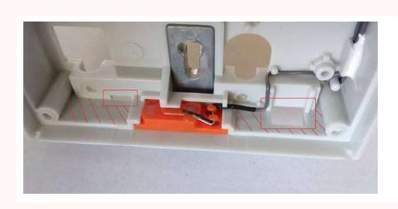
• It is forbidden to use silicone or any other sealing material on the marked and hatched places.
