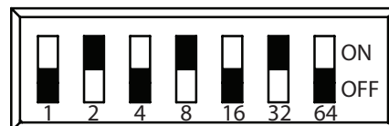
FIGURE 14: Enlarged View of PAD Device with Dip Switch Setting Addressed
