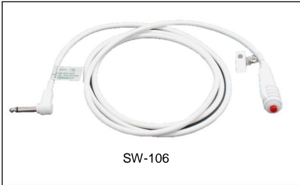
**Description:** A shockproof, plastic housing holds the cord's momentary contact push button operator, connected to a vinyl-covered cord six feet (SW-106) or ten feet (SW-110) long. The right-angle plug is molded to the cord for long life. Bedding clips are included.
