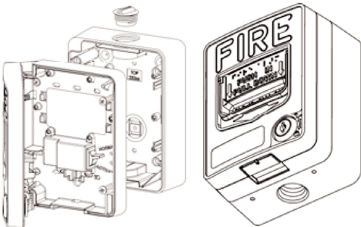
**SB-I/O shown assembled to Pull Station
