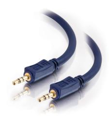
Specifically designed to provide quality music transfer from your PC sound card, portable CD player, MP3 player, iPod®, or any ministereo audio device to another audio device. This cable features two 27 AWG oxygen-free copper conductors, a drain wire, an aluminum foil shield to prevent unwanted EMI/RFI interference, and fully molded, gold-plated connectors providing strain relief for a quality connection.
