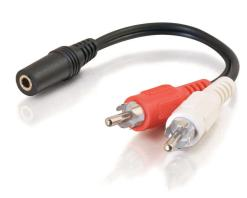
This cost-effective audio y-cable is an ideal solution for adapting your audio connections to meet your application needs. The dual conductor is shielded (26 AWG, spiral-wrapped copper shielded wire), which provides protection against EMI/RFI. The connectors are fully molded to provide excellent strain relief. Brass/nickel-plated plugs. This audio y-cable can split a signal or adapt from one connection to another.
