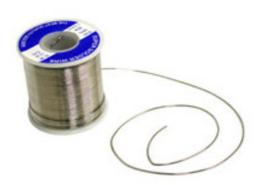
Featuring a chemistry of 99.3% tin and 0.7% copper, this lead-free solder alleviates concerns about the effects of lead on the body and on the environment. Ideal for general purpose soldering including PC board repair and tinning wires. Rosin in the solder core melts before the solder and chemically cleans the surfaces for a more reliable solder joint.
