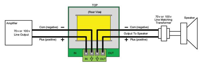
Note: Units manufactured before May 2014 had terminals located at the top. When connecting either version be sure to observe INPUT/OUTPUT and polarity designations.
