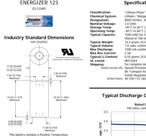
Coefficient (PTC) safety device to limit current during short circuit conditions.
