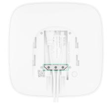
**4.** Slide ReX 2 onto the mounting panel. After installation, check the tamper status in the Ajax app and then the quality of the panel fixation. You will receive a notification if an attempt is made to tear the range extender off the surface or remove it from the mounting panel.
