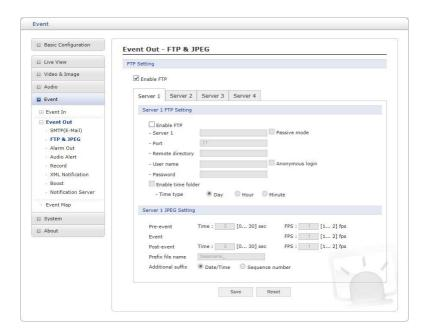
When the network camera detects an event, it can record and save images to an FTP server. Images can be sent as e-mail attachments. Check the "Enable FTP" box to enable the service. This camera can support multiple FTP servers and user can configure each server settings separately.
