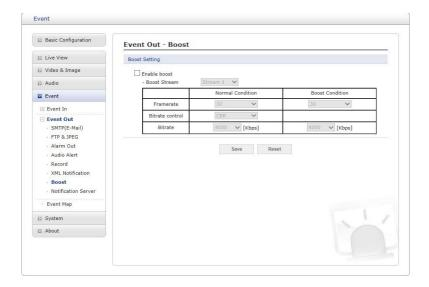
The Boost feature is used in conjunction with event detection. When this feature is turned ON, the Frame rate and Bit rate in the boost condition can be set to a different value than the ones in the normal condition field. When an event is detected, the camera will boost the Frame rate and Bit rate from the normal condition to this boosted level for the duration of the event.
