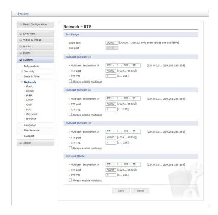
Create a setting for sending and receiving an audio or video on a real-time basis. These settings are the IP address, port number, and Time-To-Live value (TTL) to use for the media stream(s) in multicast H.264 format. Only certain IP addresses and port numbers should be used for multicast streams.
