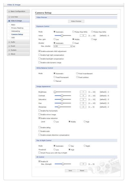
In this page, user can setup Exposure Control, White Balance Control, Image Appearance, and Day & Night control.
