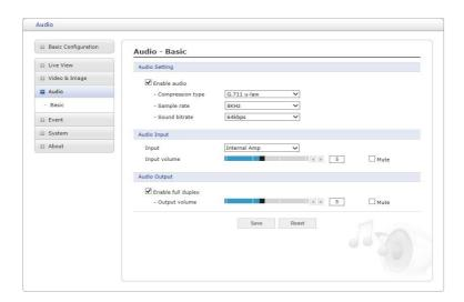
The network camera can transmit audio to other clients using an external microphone and can play audio received from other clients by attaching a speaker. The Setup page has an additional menu item called Audio, which allows different audio configurations, such as full duplex and simplex.
