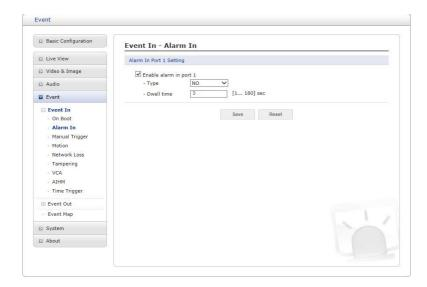
This camera provides 1 Alarm In port and user can set the port. The Port can be given as Normally Open or Normally Close state, and its Normal state can be configured. In order to use the alarm port, check the "Enable alarm port 1" first.
