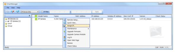
4) Select Assign IP Address. The Assign IP window will display. Enter the required IP address.
