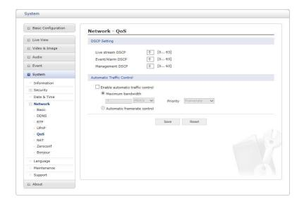
Quality of Service (QoS) provides the means to guarantee a certain level of a specified re-source to selected traffic on a network. Quality can be defined as a maintained level of bandwidth, low latency, and no packet losses.
