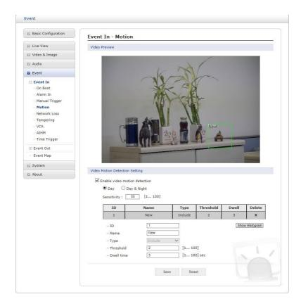
This option makes use of the motion detection function with 16 programmable areas, 8 **Include** and **Exclude** zones each.
