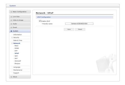
The network camera includes support for UPnP. UPnP is enabled by default, so the network camera is automatically detected by operating systems and clients that support this protocol. Enter a name in the Friendly name field.
