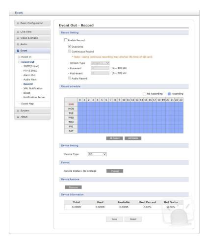
When the network camera detects an event, it can record the video stream onto the Micro SD Memory (not supplied) or NAS (Network Attached Device) as a storage device. Check the "Enable Record" box to enable the service.
