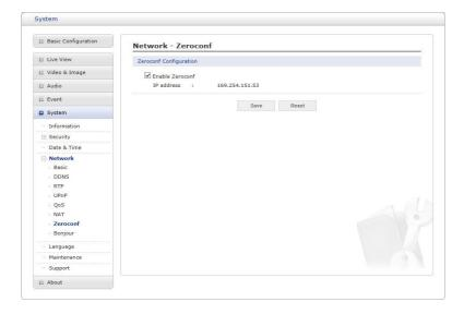
Zero configuration networking (zeroconf) is a set of techniques that automatically creates a usable Internet Protocol (IP) network without manual operator intervention or special configuration servers.
