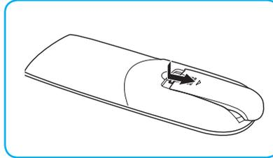
2. Install new batteries (AAA). Ensure that you have the batteries' polarity (+/-) aligned correctly.
