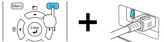
4. When the On/Standby and Status lights are blue, and the Laser and Temp lights are orange, release the **Esc** button.
