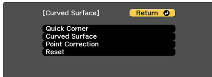
**Note:** You can also access the **Curved Surface** setting by pressing the **Menu** button and selecting **Geometry Correction** on the Settings menu.
