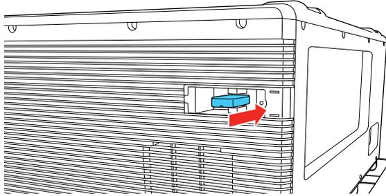
4. Replace the wireless LAN module port cover.
