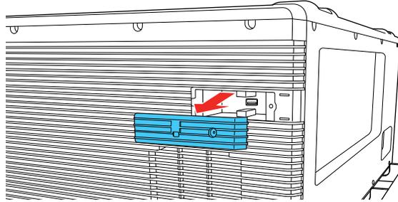
4. Make sure the wireless LAN module is installed in your projector.
