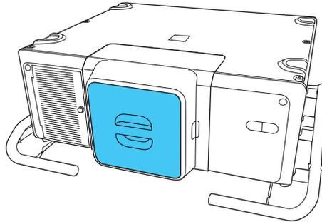
3. To lift or lower the projector, install four commercially available eye bolt screws to the screw thread holes in each corner of the projector or to the handle. Attach straps or chains to the screws and make sure the angle of the strap is 60 degrees or more when lifting or lowering the projector.
