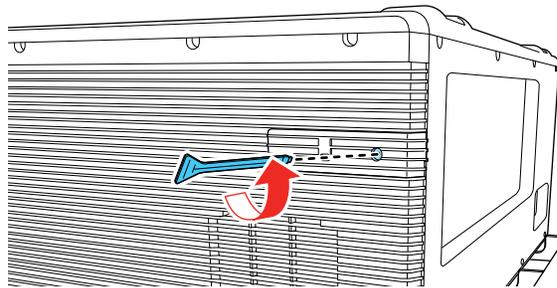
2. Remove the wireless LAN module port cover.
