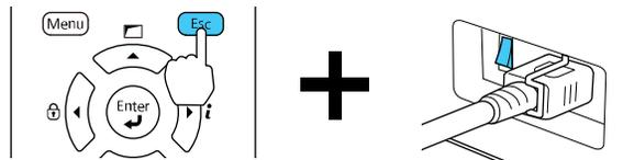
5. When the On/Standby and Status lights are blue, and the Laser and Temp lights are orange, release the **Esc** button.
