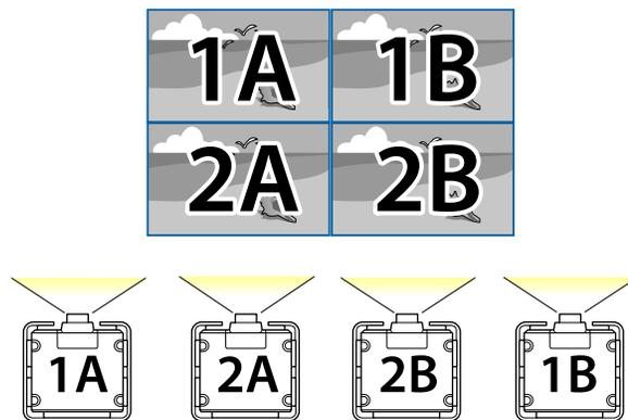
**Note:** Before tiling, make sure the displayed images from your projectors are rectangular, correctly sized, and focused.
