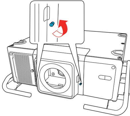
3. Press the tabs on both sides of the lens cover and pull the lens cover off the projector.
