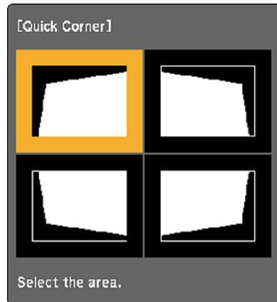
**Note:** You can also access the **Quick Corner** setting by pressing the **Menu** button and selecting **Geometry Correction** on the Settings menu.
