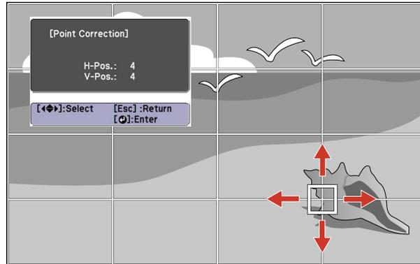
8. Press the arrow buttons to correct the image shape in all necessary directions.
