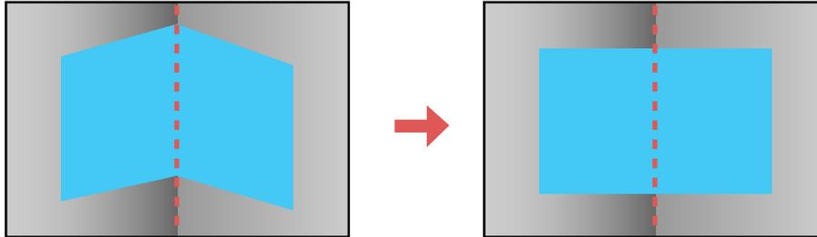
**Note:** For the best results, project from the front of the screen onto a right-angled surface. The image may not be evenly focused throughout even after performing the steps here.
