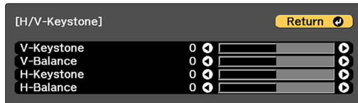
**Note:** You can also access the **H/V Keystone** setting by pressing the **Menu** button and selecting **Geometry Correction** on the Settings menu.
