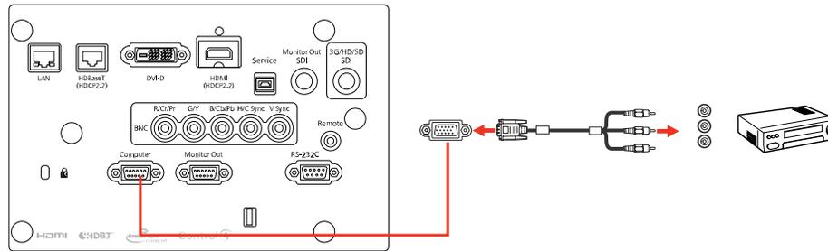
3. Tighten the screws on the VGA connector.
