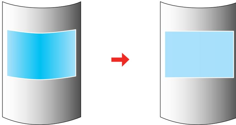
**Note:** For the best results, project from the front of the screen onto a surface with a uniform arc radius and with the lens in the home position.
