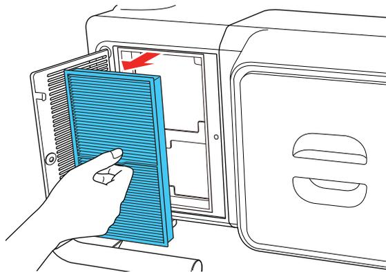
5. Tap each side of the air filter 4 to 5 times to shake off any excess dust.
