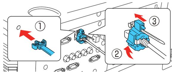
3. Place the open cable clip around the HDMI cable, but don't lock it into place.
