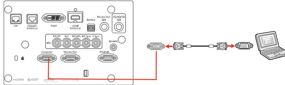
4. Tighten the screws on the VGA connector.
