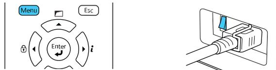
5. When the On/Standby and Status lights are blue, and the Laser and Temp lights are orange, release the **Menu** button.
