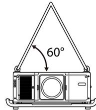
**Caution:** Do not use the eye bolt screws for permanent installation as this can cause damage.
