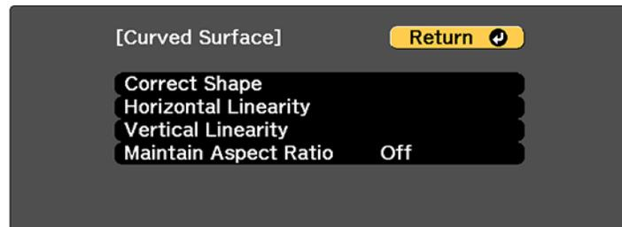
11. To compensate for expansion or contraction while maintaining the image aspect ratio, select **Maintain Aspect Ratio** and set it to **On**.
