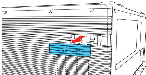
3. Insert the wireless LAN module into the port.
