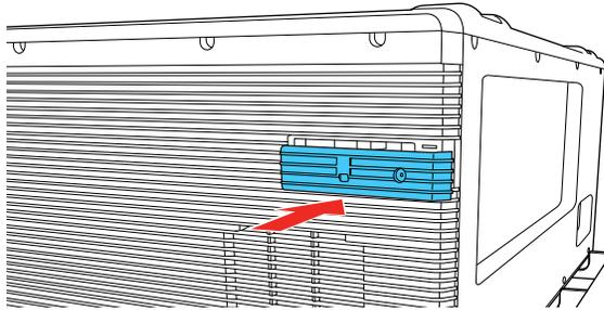
5. Secure the wireless LAN module port cover using the screw you removed.
