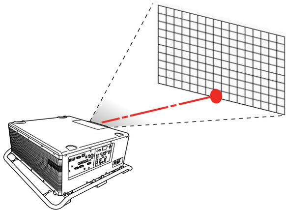
**Note:** You can also press the **Focus +** or **-** button on the remote control to focus the center of your image. Then use the **Distortion +** or **-** button to adjust the edges of the image.
