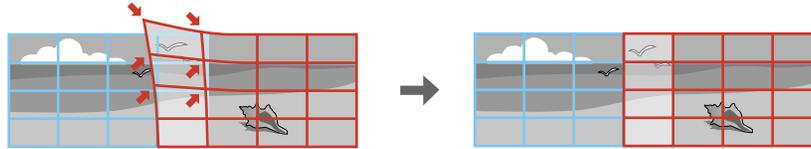
**Note:** You can move the points on the grid between 0.5 to 32 pixels in any direction. Coordinates for pixels that extend beyond the edge of the projected screen are displayed as negative numbers.
