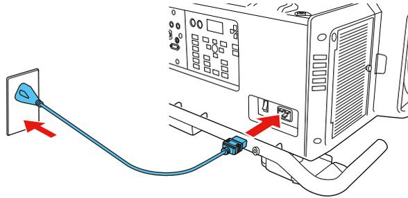
**Note:** If you connected the projector using the 120 V power cord, the image brightness is reduced to approximately 30% of the brightness achievable with the 220 V power cord and the Laser light flashes orange. For optimal performance, connect the 220 V power cord that came with the projector. You cannot use the **Light Source Mode**, **Estimated Remains**, **Refresh Mode**, or **Light Source Calibration** functions when connected using the 120 V power cord.
