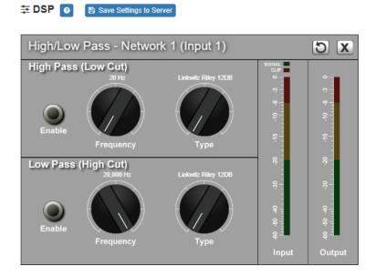
Figure 12, High/Low Pass Parameters
