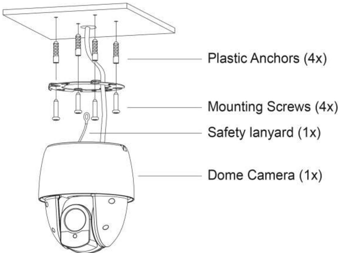
**CAUTION: A silicone rubber sealant must be applied to seal the housing to secure waterproofing.**
