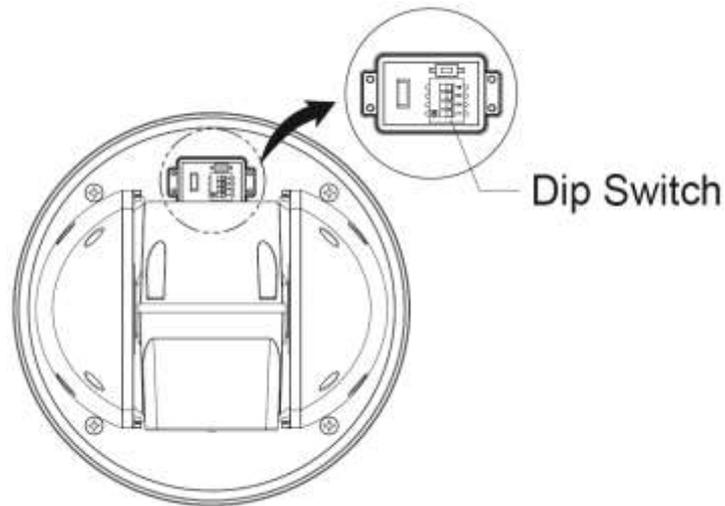
**NOTE:** Open the DIP switch cover and change the setting of DIP switch.
