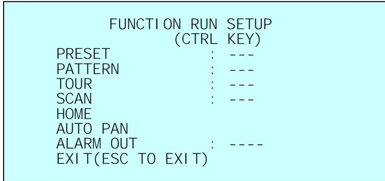
1. Select the desired Function by pressing the **Up** or **Down** key.
