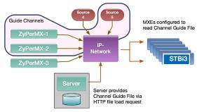
In the diagram shown, if the guide file is specified as exclusive, and the only entries in that guide file are for ZyPerMX-1, ZyPerMX-2, and Source 5, then any other channel will be ignored and not included in the guide. The only stream the user will be able to select are for the channels described in the guide file.
