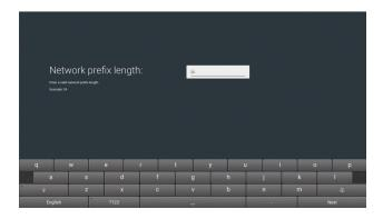
Network prefix length sets the network subnet mask. A setting of 24 is equivalent to setting the mask to 255.255.255.0
