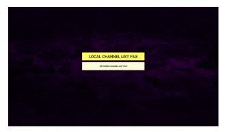
In the dialog, enter the pointer to the location on the web server where you have placed the Channel Guide file. Local Channel List File would be located on a USB memory stick plugged into on of the STBi3 USB ports. The location of a Network Channel List file depends on where the IT admin has allowed HTTP file browsing to.
