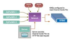
If the guide file is in "Additive" mode only the non-ZeeVee channels need to be specified in the guide file. The ZeeVee channels will send beacons that are learned by the STBi3 and those channels will automatically be added to the guide. In the diagram shown Source4 and Source5 are streams supplied by non-ZeeVee equipment. Only stream information for Source 4, and Source 5 need to be specified in the guide file.
