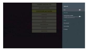
If a DHCP server is on the network, the IP address and associated fields will automatically be filled in. Otherwise the fields must be manually entered. Scroll down to IP setting and click the OK button on the remote. Then choose static
