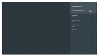
Note: Auto select will read display EDID to set resolution. Manually selecting a resolution not supported by the display can result in loss of image.
