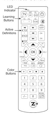
The STBi3 decoder is supplied with a partial learning remote control device. Buttons P1-P5 can be programmed to mimic the functions of a select set of buttons from another remote control unit
