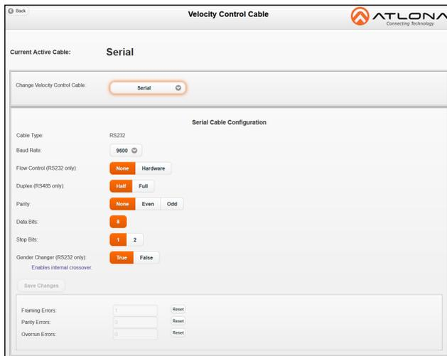
**NOTE:** The RS-232 parameters should match the controlled device. Verify the parameters using the source or display's manual.
