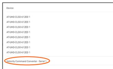
Velocity will automatically set the Velocity Command Converter to the correct baud parameters when the save button is pressed.
