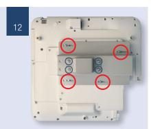
Carefully place the projector plate on top of the spacers and washers and secure the plate with  $4 \times 4$  allen head screws M4  $\times 20 \times 4$  (0.15"  $\times 1 \times 4$ ").
