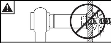
ENG Do not overtighten screws.
