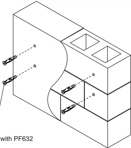
concrete anchors provided with PF632
