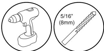
ENG Drill mounting holes into supporting surface (2.5" (64mm) minimum depth required).
