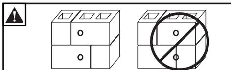
ENG Do not drill into mortar joints.
