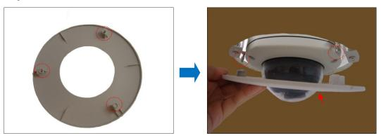
2. Push to firmly secure the flush mount cover latches.
