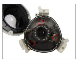
CAUTION: When using electric screwdrivers, be careful not to touch the internal camera components while attaching the screws. Since electric screwdrivers vary in sizes, speed, and force, they may bruise and damage the internal camera components.
