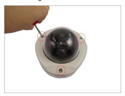
4. Carefully lift to open the dome cover and place it on the side of the camera.
