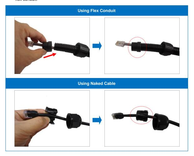
4. Pull the network cable through the camera conduit hole.
