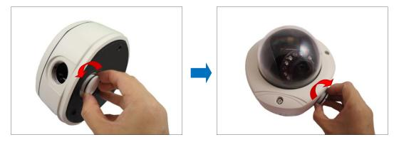
3. Loosen the three (3) screws securing the dome cover.
