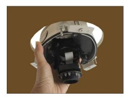
2. Position the retaining brackets to hold the mount on the ceiling.
