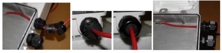
Insert sleeve with the cable attached into cable gland & box. Screw top on; be sure correct amount of cable is inserted into the sleeve to connect to board before you tighten the top. When top of cable gland is tight connection is very weather resistant.
