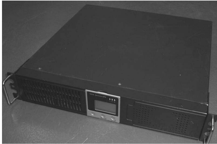
UPS FRONT VIEW AFTER INSTALLING 2U EARS
