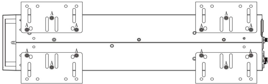
SX-BDL-2000 / UPS-2000-OL / UPS-3000-OL Use M4 x 6 screws on places marked with letter A
