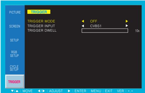
Default setting is OFF and switch to ON trigger mode
