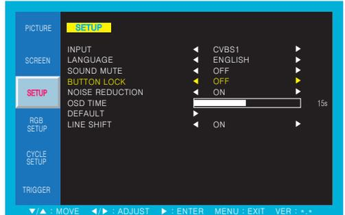
Default setting is OFF and switch to ON button lock option
