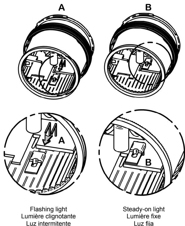
Each module can have a **steady-on** or **flashing** function, by keeping or removing the jumper on the circuit.
