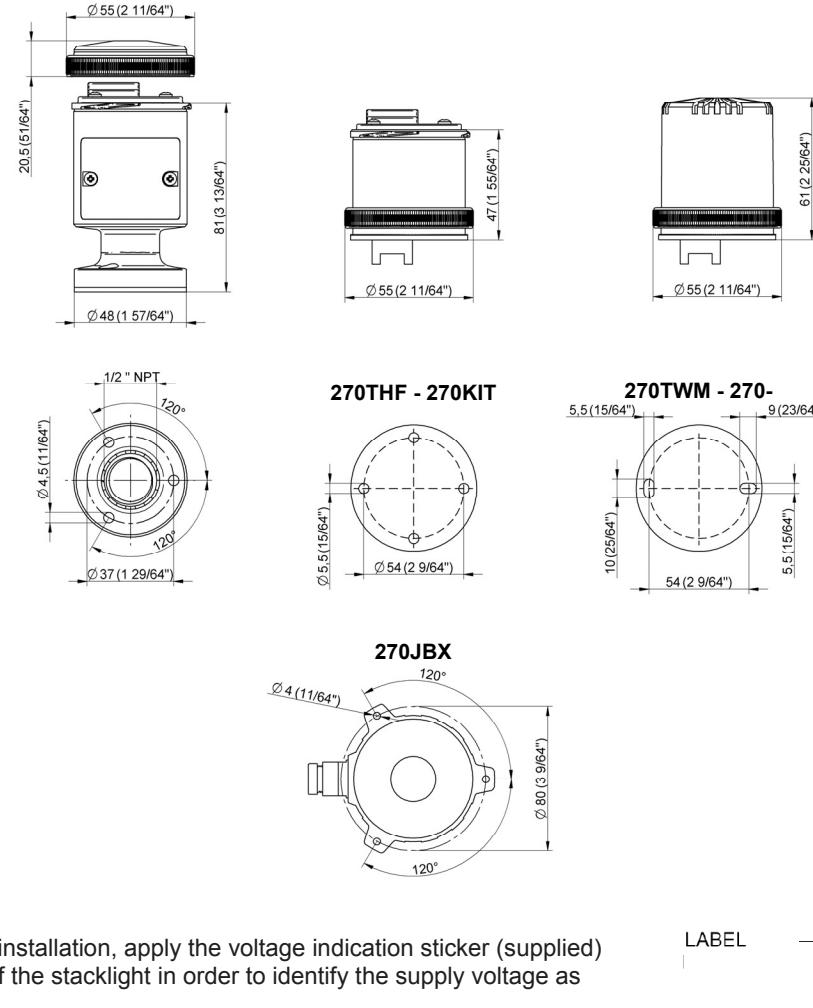
**Important:** at the time of installation, apply the voltage indication sticker (supplied) to the label on the base of the stacklight in order to identify the supply voltage as indicated in the drawing
