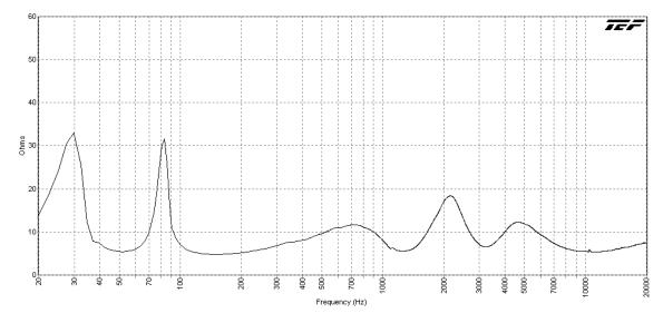
AH94-8ST Impedance (ohms) vs. Frequency
