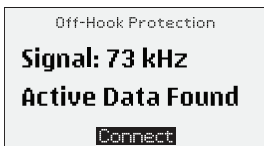
Figure 4.4 Data Present Warning
