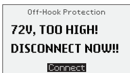
Figure 4.1 Over Voltage Warning
