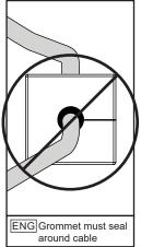
ENG Slide grommets into enclosure, aligning grooves of grommet with grooves in cable gland.
