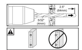
ENG Mounting hole must center on stud.
