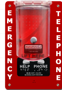
RCB2100NRCOV Red Fiberglass NEMA 4 Rated Outdoor Surface Call Box with Protective Cover O.D. : 6.60"W X 9.90"H X 3.25"D (mm: 168 W X 251 H X 83 D) Cover: 3.75"W X 6.40"H X 2.25"D (mm: 95W X 163 H X 57.15 D)
