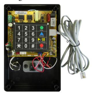
\*Use 22 or 24 AWG 2-pair twisted, shielded cable between the phones and the SmartRescue. The maximum communication run is 5,100'
