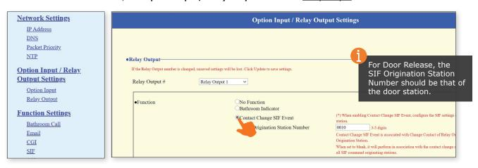
Starting with Relay Output 1, select Contact Change SIF Event and then specify the Station Number of the station activating the Relay Output 1. Once these values are set, click **Update**. Depending on the browser, the IXW-MA may return to the login screen which Update is selected.
