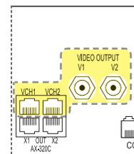
The AX-084C and AX-248C both have the ability to connect to the AX-320C add-on unit. Connect the X1 and X2 with two CAT-5e cables. Both X1 and X2 must be connected and the AX-320C must be within 16 feet of the main CEU.
