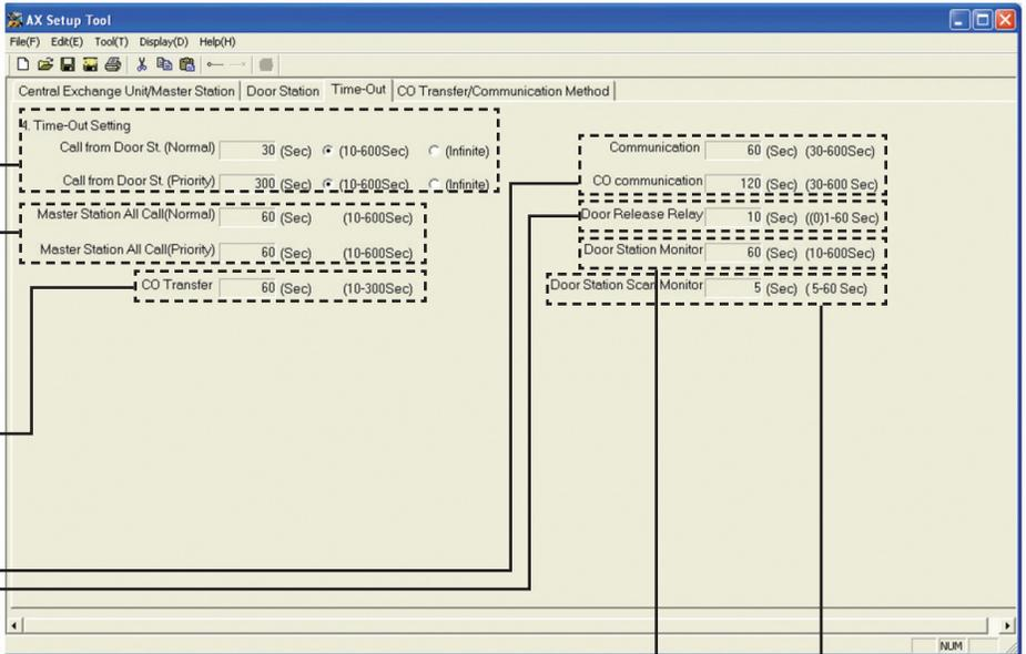
Step 6: Set the Door Station Monitor for the amount of time that you want to be able to listen in to a door station (10 to 600 seconds). When a door station is selected, the master will be in listen mode for this length of time, then will time out..
