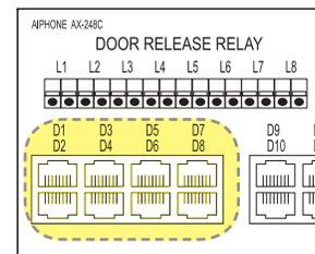
The Door Release Contacts can be individually programmed to be either N/O or N/C. The contacts are located above the door station ports. "L1" are the contacts\* for door station port "D1", "L2" are the contacts for "D2", etc. As the "L#" connections are dry contacts, a separate power source is required for the actual door strikes or magnetic locks.
