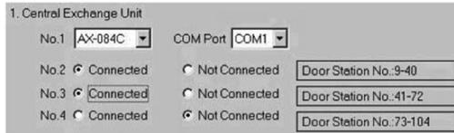
The screenshot shows the configuration interface for the Central Exchange Unit. It includes a title bar '1. Central Exchange Unit', a dropdown menu for 'No.1' set to 'AX-084C', and a dropdown menu for 'COM Port' set to 'COM1'. Below these are three rows of radio button options for 'No.2', 'No.3', and 'No.4'. Each row has 'Connected' and 'Not Connected' options. To the right of each row is a text box for 'Door Station No.' with values '9-40', '41-72', and '73-104' respectively.
