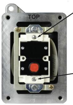
LOOSEN THIS SCREW TO REMOVE SWITCH BLOCK
