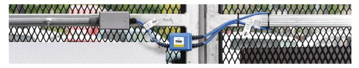
Be sure to avoid installing the cable in such a way that the cable will move back and forth against a sharp metal edge causing abrasion. We do not recommend installing in the pipe frame unless a rubber grommet or similar guard can surround the cable where it meets the metal.
