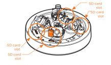
3. To remove the SD card, press the card gently into the card slot to release it. The card will pop out automatically.
