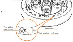
**Resetting the camera:** To reset the camera, use the tip of a paper clip or a pencil and press the reset button. Pressing the button for five (5) seconds will initiate a camera-wide reset of all the settings, including network settings.
