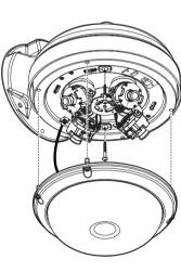
4. Adjust the camera modules on the magnetic surface. Each camera module snaps into position using the magnetic track. Use the diagram below to properly align the modules.
