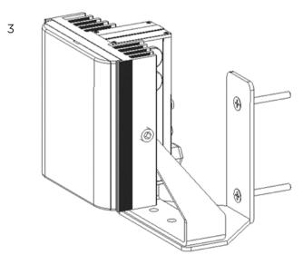
With the bracket secured to the wall, attach the illuminator with the supplied M6 nuts and bolts. Attach the center bolt first then rotate the illuminator to the required horizontal position. Once the necessary position is achieved, secure the illuminator the remaining nut and bolt in one of the outer holes.
